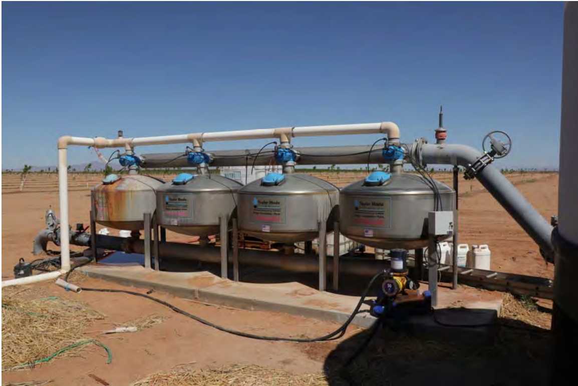
Drip irrigation filtration system
